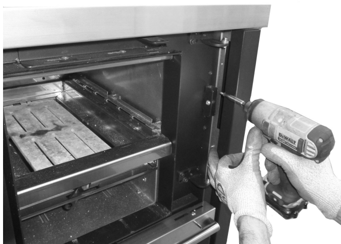
Fig. 27 - Retirer le support
